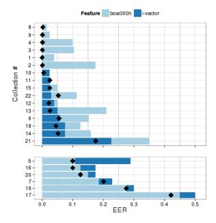
**Fig. 3.** Impact of lexical, non-lexical and fusion on individual collections, ordered by best performing feature. Bar endpoints indicate individual feature EER for i-vectors and 300h bags-of-words, with the dot indicating the performance from score fusion of the two.
